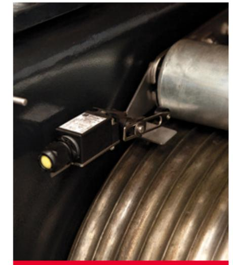
**Slack Rope Limit Switch & Rope Guide**
