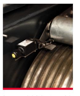
**Slack Rope Limit Switch & Rope Guide**
