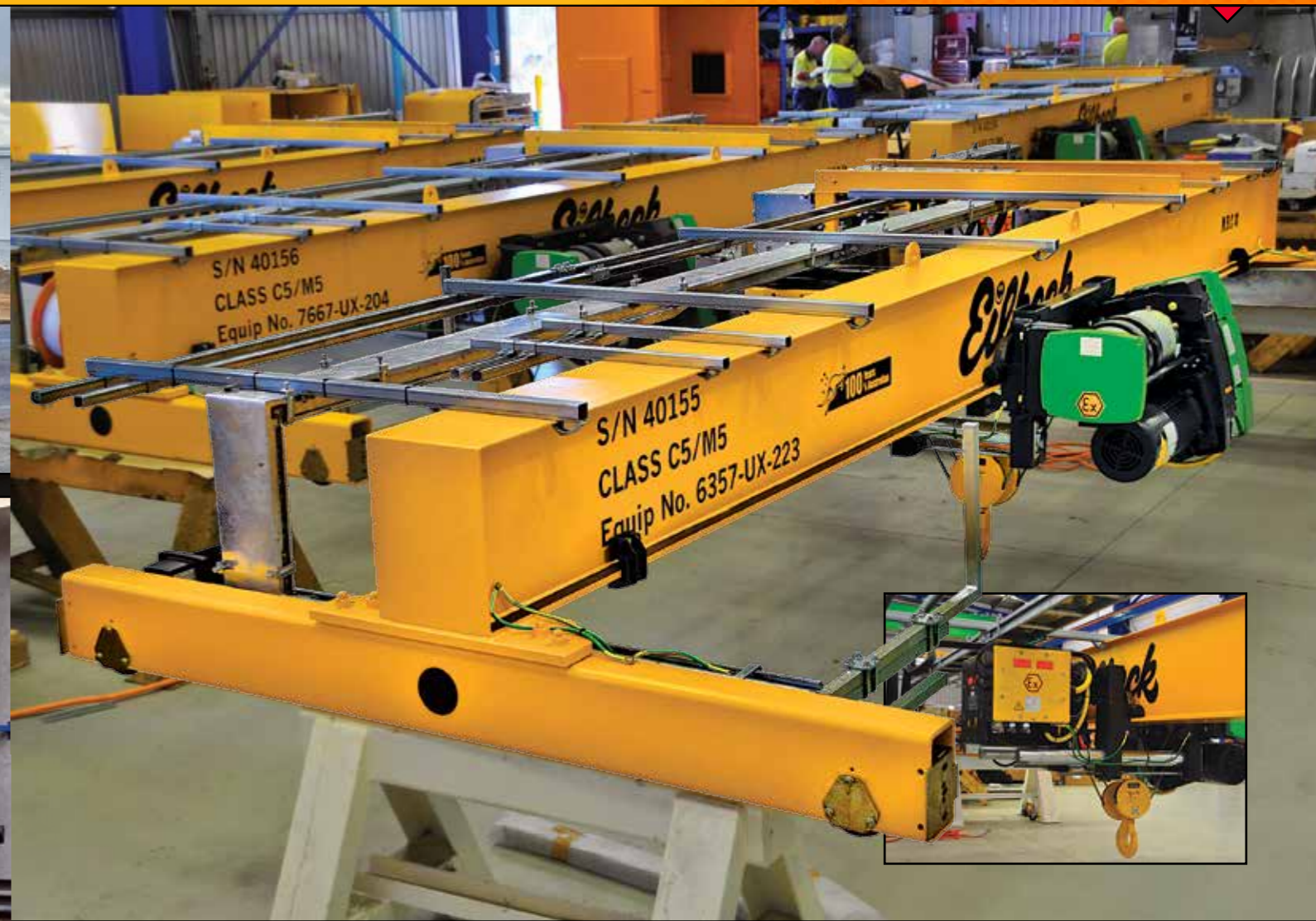
5t ZLK Crane for Main Sub-station, Ichthys Onshore LNG Facilities Project
