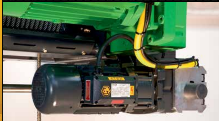
Motors made of grey cast iron and IP 66 rated, the type of protection combines flameproof enclosure, increased safety and protection by housing
