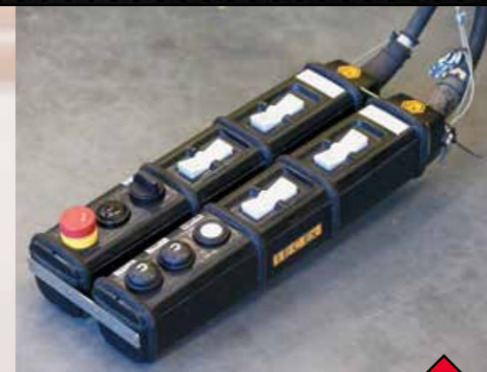
Control Pendant Flameproof Housing Protection IP 66
