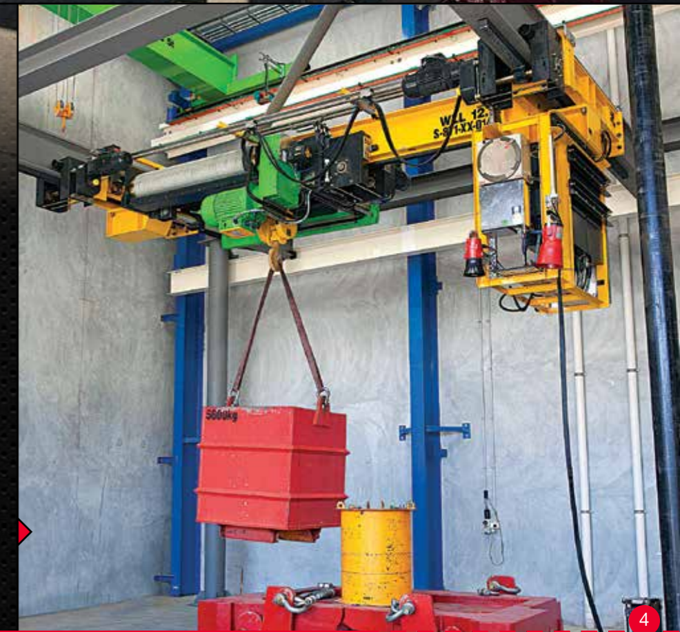
27.5t FPSO Ex Crane under load testing
