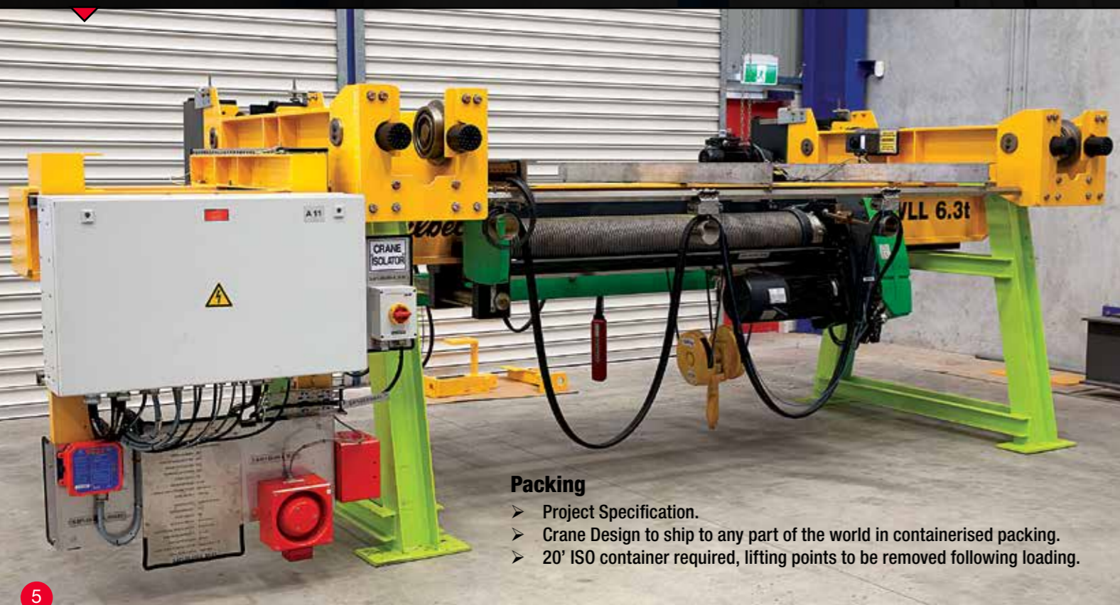
Single Girder 6.3t ELD Crane with shipping support frame for INPEX Ichthys Project
